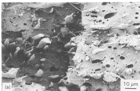
Figure 12 Scanning electron micrographs of a fractured surface of 75/25 PPS/LCP blend: (a) skin region; (b) core region.
