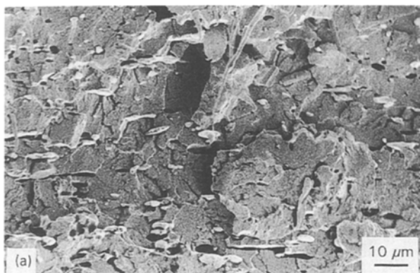
Figure 11 Scanning electron micrographs of a fractured surface of 90/10 PPS/LCP blend: (a) skin region; (b) core region.
